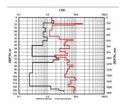
Comparisons of the DCP test results before and after injection showed a 699% improvement in the California Bearing Ratio (CBR) between the treated depths of 3 to 10 feet at the first location and a 277% improvement at the second location.
